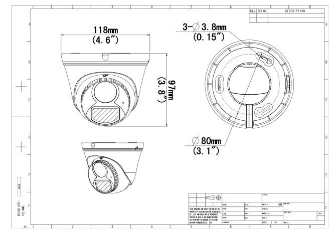
Aggregate product size diagram using UAC-T115-AF28-DL as an example
