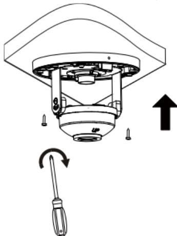
4. Adjust the monitoring direction of the lens (tighten screws after vertically adjusting the lens).
