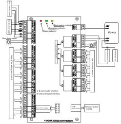
Pay attention to the format selection of the when connecting to the access controller, the WEGAND26/34 card reader, WEGAND26/34 line is grounded by default The corresponding status of indicators are illustrated as follows.
