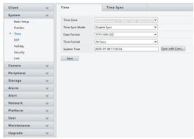
Choose the time zone, time sync mode, date format, and time format as needed. Then set the system time manually.
