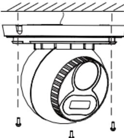
5. Mount your camera. Mount the housing with install mark aligned.
