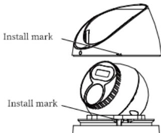
4. Install the base plate and the camera. Connect cable and protect it with waterproof tape and attach dome to ceiling with taping screws.
