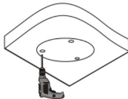
2. Lead the cables out from the ceiling. Knock the plastic anchors into the guide holes and ensure that they are tightened up.
