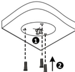
3. Detach the housing from the base plate with the marks aligned.
