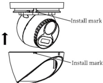
6. Adjust the monitoring direction. Rotate the camera to desired monitoring direction.
