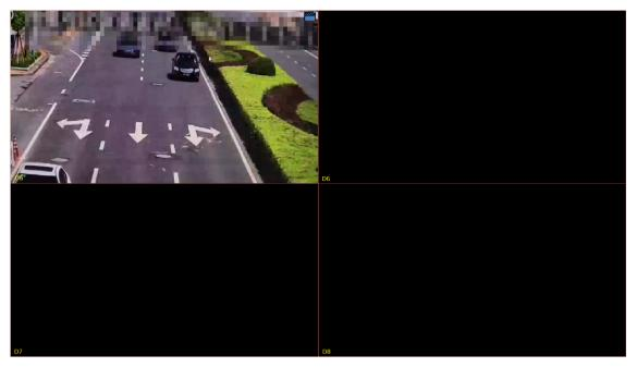
• When Max. Alarm-Triggered Live View Windows is set to 9 Windows, the live view page plays the live video of each camera in 9-split mode. If more than 9 cameras are linked, the live video switches at 5s.
