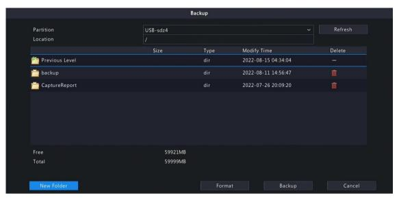
6. Select the partition and storage path, and then click **Backup**. The snapshots are saved in the specified path on the storage device. You can also create a new folder for the snapshot(s) by clicking **New Folder**.
