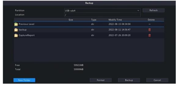
6. Select the partition and storage path, click **Backup**. Then the recordings are saved to the specified path on the storage device. You can also create a new folder for the recording(s) by clicking **New Folder**.
