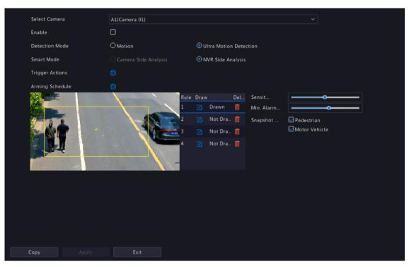
2. Set detection rules. The 4 detection rules shall be set separately. The following takes Rule 1 as an example.
