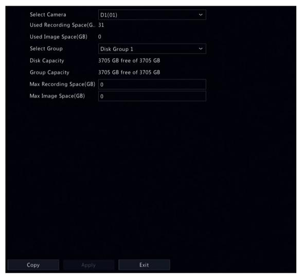
2. Select a camera, select a disk group for storage by the camera, and allocate storage space for videos and images from this camera on the disk group.
