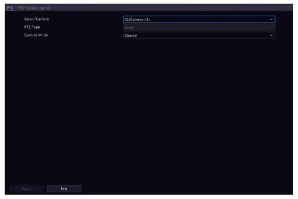
2. Choose a control mode according to camera connection method, and complete other settings.
