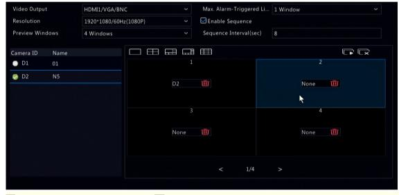
Note: On the left-side channel list, [ ] is empty for D1, which means the channel is not bound to any window.
