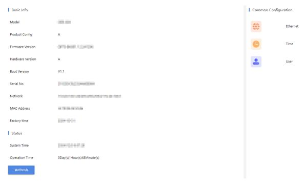
Common Configuration: Click the icon or text to quickly access the common functions, including Ethernet, Time, and User
