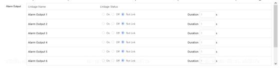
When Linkage Status is set to On, you must set the alarm output duration.
