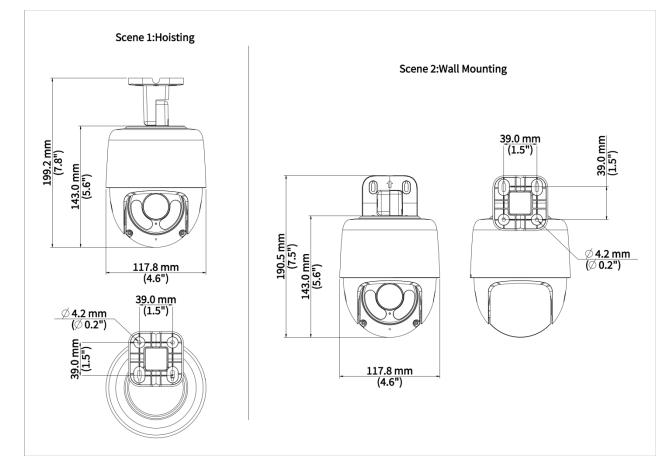
Aggregate product size diagram using "main model" as an example
