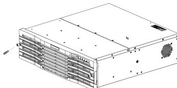
2. Fix the tray that comes with the rack to the rack. Ensure that the tray's support surface aligns with the "U" scale on the rack's square hole rail.
