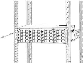
5. Install the front panel to complete the installation.
