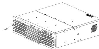
3. Align the disk with the disk slot and then gently insert the disk.
