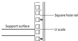
3. Push the device along the tray into the rack, ensuring it is flush with the square hole rails.
