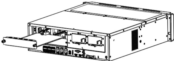
3. Fasten the screws of the expansion card.
