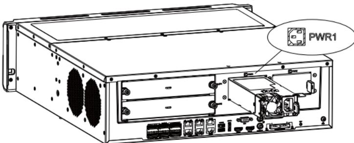
3. Complete the power module installation.
