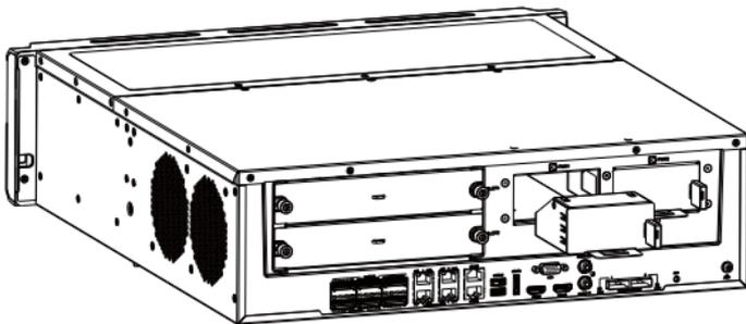
2. If there is a power silkscreen on the device, you can confirm the direction of the power interface according to the silkscreen. If there is no silk screen, insert the power module in the direction as shown in the figure below.
