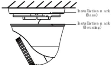
6. Adjust the monitoring direction. The camera can pan 360° and tilt 75°.
