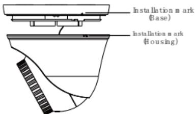
4. Lead the tail cable through the base. Then mount the base onto the ceiling using self-tapping screws.
