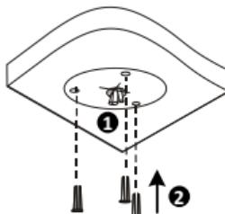
3. Rotate the housing till the marks are aligned, detach the housing.
