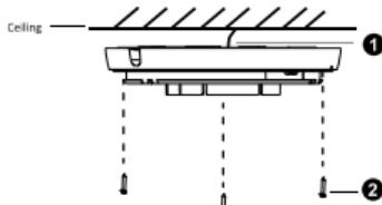
5. Connect all cables and take waterproof measures. Align the installation marks, attach the housing to the base, and then rotate to fasten.
