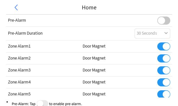
After **Pre-Alarm** is enabled, when you switch the arming scene on the screen, a sound will be played and the message "**Pre-alarming...**" will be displayed as the set pre-alarm duration.
