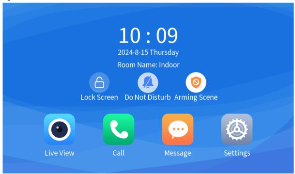
The home screen displays the current time (set on the Web), and supports Lock Screen Manually, Do Not Disturb, Arming, Live View, Make Calls, Answer Calls, Message, and Settings.
