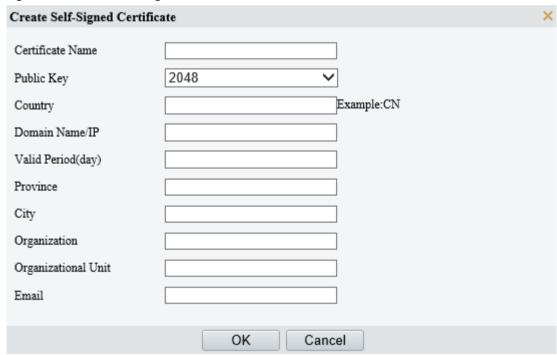
• Certificate: It is used to apply the self-signed certificate or imported certificate to be a CA certificate, which is suitable for application scenarios with high security requirements.
