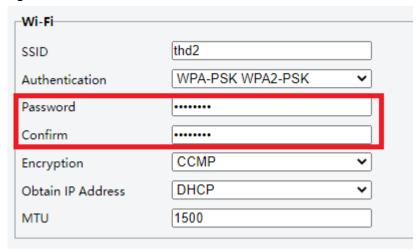
5. Click **Save**. Wait about 3 seconds, and then the **Network Status** tab displays the current network status of connected Wi-Fi.
