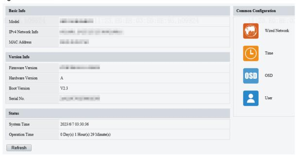
Common Configuration: Click the icon or text to quickly access the four common functions, including Wired Network, Time, OSD, and User.
