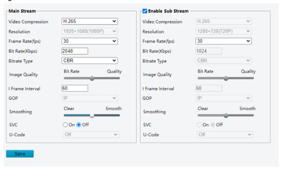
2. Set the main stream parameters. The following introduces some parameters.
