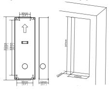
(2) Keep the recess bracket facing outward and upward, and insert four pointed tail cross screws into inside holes to secure the bracket on the wall.
