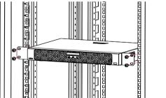
4. Insert the screws into the holes and tighten the screws using a screwdriver.
