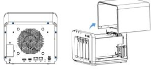
2. Loosen the screw on the PCIe filler panel, remove the filler panel.
