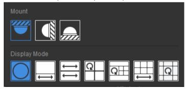
Choose the correct mounting mode for the fisheye camera: ceiling, wall or desktop, and then display modes appear, e.g., 360° Panoramic, 180° Panoramic, Fisheye, PTZ (appears when the pointer rests on it). Display modes and operations supported vary with mounting mode.
