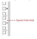
3. Align the mounting bracket holes with the floating nut holes, and place the device on the rack.
